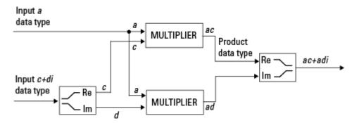
**Complex-Complex Multiplication.** The following diagram shows the multiplication of two complex fixed-point numbers. Note that the software returns the output of this operation in the sum data type, which is governed by the fimath object SumMode property. The intermediate product data type is determined by the fimath object ProductMode property.
