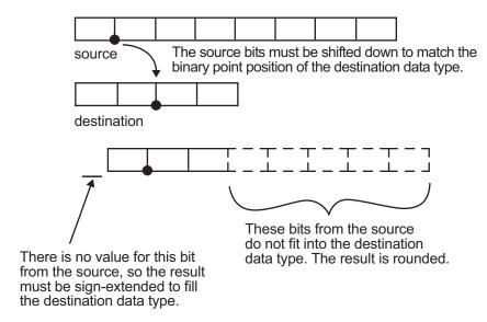
As the diagram shows, the source bits are shifted down so that the binary point matches the destination binary point position. There is no value for the highest bit from the source, so the result is sign-extended to fill the integer portion of the destination data type. The bottom five bits of the source do not fit into the fraction length of the destination. Therefore, precision can be lost as the result is rounded.
